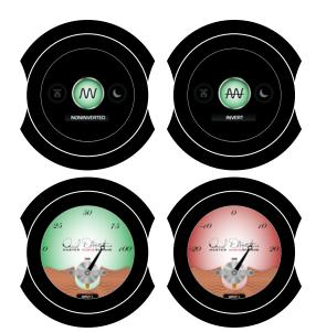
red when the polarity is inverted.
